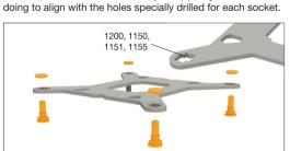
For fixing the backplate screws onto the Intel backplate use the O-rings. Once assembly of the Intel backplate for the respective Intel socket is complete, position it under the motherboard. In so doing make sure that the Intel backplate screws are precisely positioned inside the motherboard holes.
