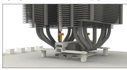
Fasten the Silent Wings 3 120mm fan using fan clips onto the front side of the cooler. Slide the 135mm fan between the two heatsinks and also fasten this with fan clips. Connect both fans using the the Y cable. Connect this to the CPU fan connector on the motherboard.
