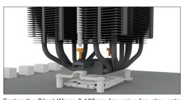
Fasten the Silent Wings 3 120mm fan using fan clips onto the front side of the cooler. Slide the 135mm fan between the two heatsinks and also fasten this with fan clips. Connect both fans using the Y cable. Connect this to the CPU fan connector on the motherboard.
